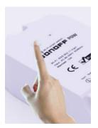
2. Press the button for 7 seconds until the green LED blinks like this: blinks 3 times and on repeatedly:
